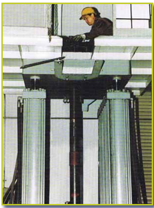
Petroleum Casing Tensile Test
